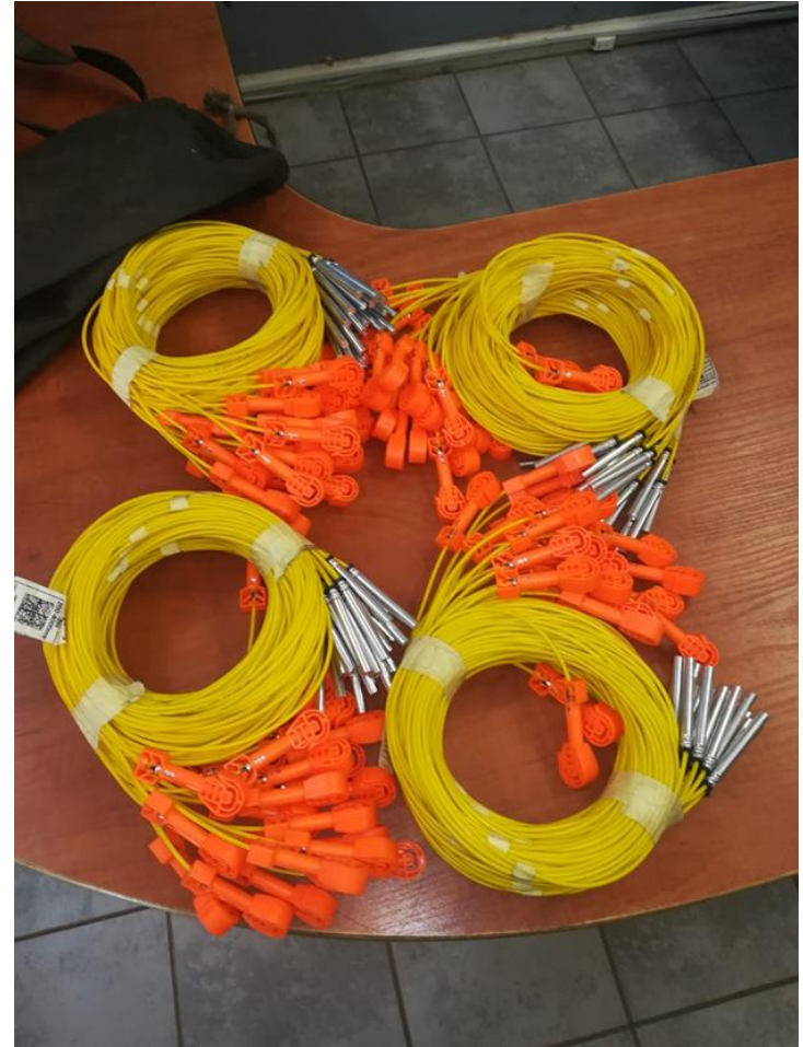
Shock tube assemblies found in possession of an underground miner returning to surface after his shift
